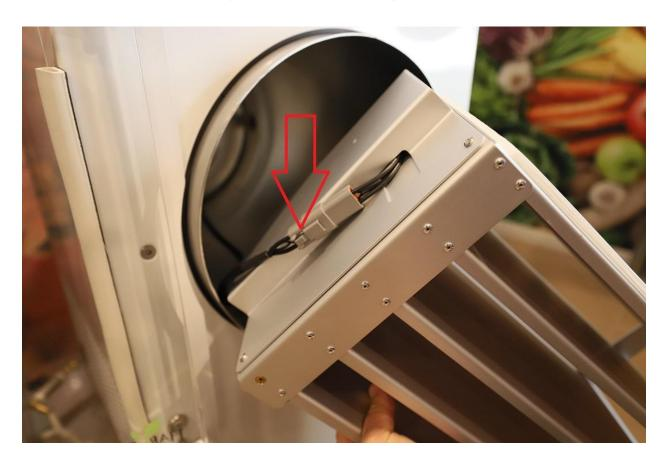
Put the gasket back on, close the door and make sure that it is getting good contact, and ensure that the pump is plugged into the outlet on the freeze dryer and pump switch is at the "on" position. Make sure that your pump has clean, fresh oil as well. The oil in the pump serves many purposes other than lubrication. It also helps seal parts and pieces for vacuum. (as mentioned earlier)
