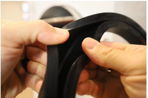
You can also run a cotton swab or other cleaning tool in the back crevice of the gasket several times to determine if there is an obstruction or debris. This gasket is the easiest place for vacuum to escape so it is best to clean this frequently. The best type of cleaner for all parts of the freeze dryer is soap and water. Check the front of the gasket as well and clean if needed.
