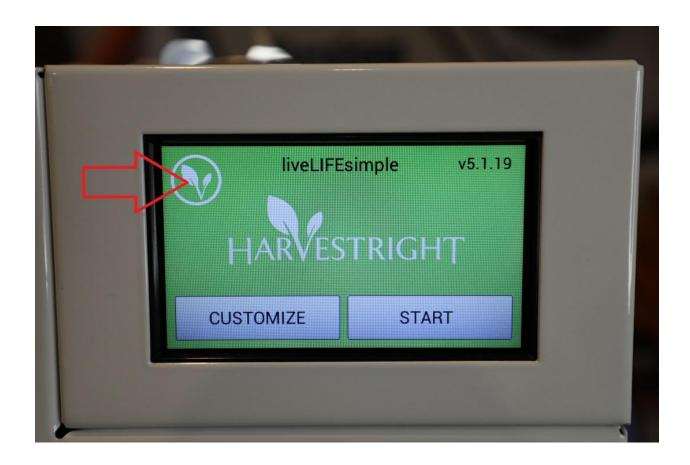
(If you have an older version of Freeze dryer, you may not have this option.) If you have older software, you can press TEST and manually turn on the vacuum from there. If your Harvest Right is even older, you may not have the ability at all. However, you can still plug your vacuum pump into a wall outlet and do this manually.
