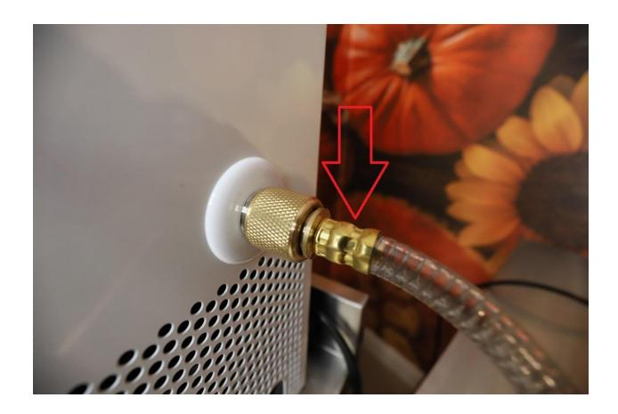
If you suspect that this is the problem, Harvest right can sell or provide you with a new hose or you can use self fusing silicone tape to wrap the crimps. This can be found at any hardware store.
