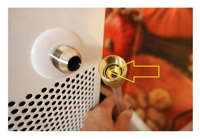
If there is debris, damage or a break, replace the O-ring. They can be found at any hardware store.
