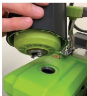
FIGURE 7: Demister removed, showing oil opening
