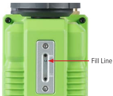
FIGURE 8: Sight glass, showing oil level. NOTE: When the pump is running, the oil level in the sight glass will drop slightly
